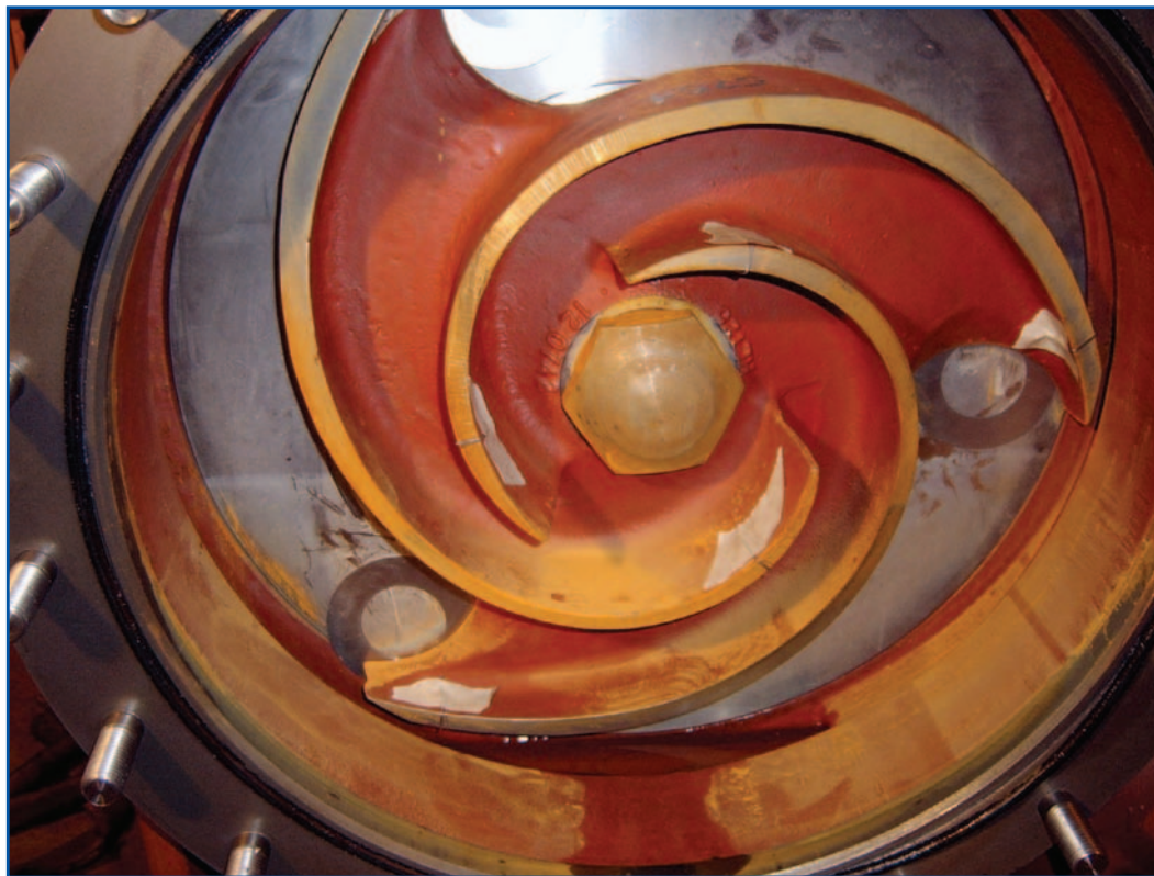
The heart of the beast – the massive 508 mm impeller is the heart and soul of the new HL130M and HL160M Godwin high head pumps. A single impeller is now delivering heads to 183 m with flows up to 350 m 3 /hr.
